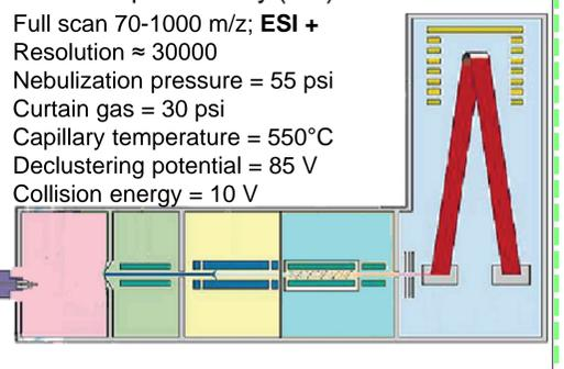
Fig. 2. A schematic representation and main parameters of LC-QTOF defined method.
